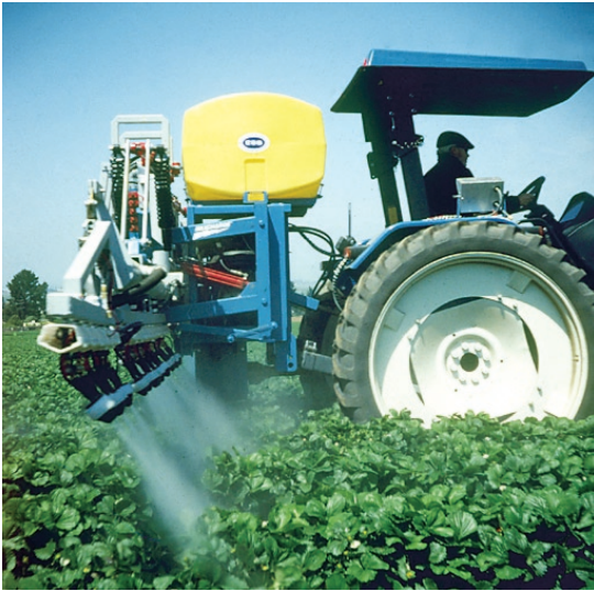
ESS air-assisted electrostatic sprayers allow you to cover an average of 30 or more acres per 150 gallon tank of chemical. Compare this to the 500 gallon tank on most hydraulic sprayers.
