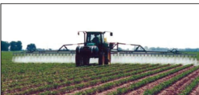
The K-450 Series is available with 40 to 72 nozzles on booms from 36 to 66 feet in length.
