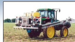
The K-450 Series is available with 40 to 72 nozzles on booms from 36 to 66 feet in length.
